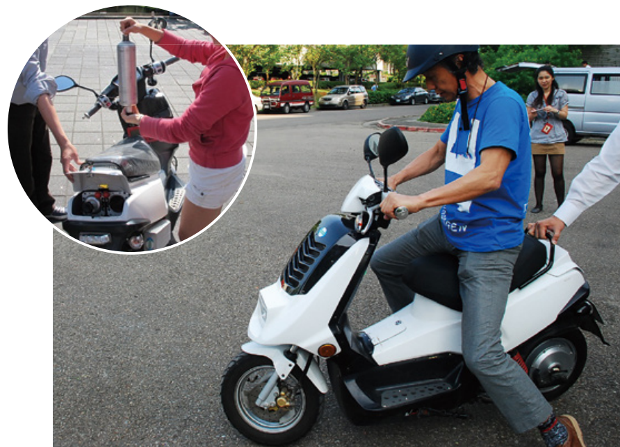
A fuel cell scooter developed in Taiwan. Hydrogen is charged by changing the metal hydride cartridges. The scooter's range with two cartridges is approximately 80 km. Each cartridge holds 45 g of hydrogen.
