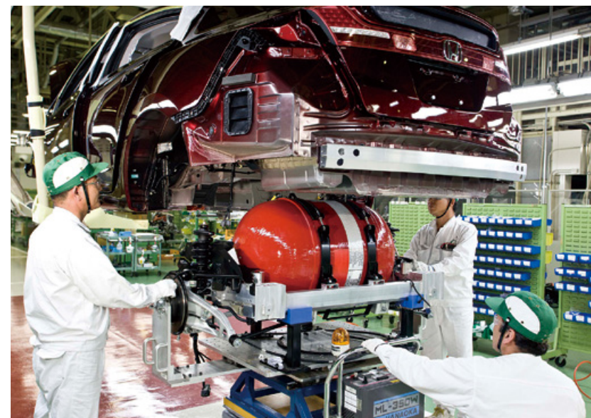
Hydrogen tank loading process in the FCX Clarity, Honda's fuel cell vehicle (June 2008).
