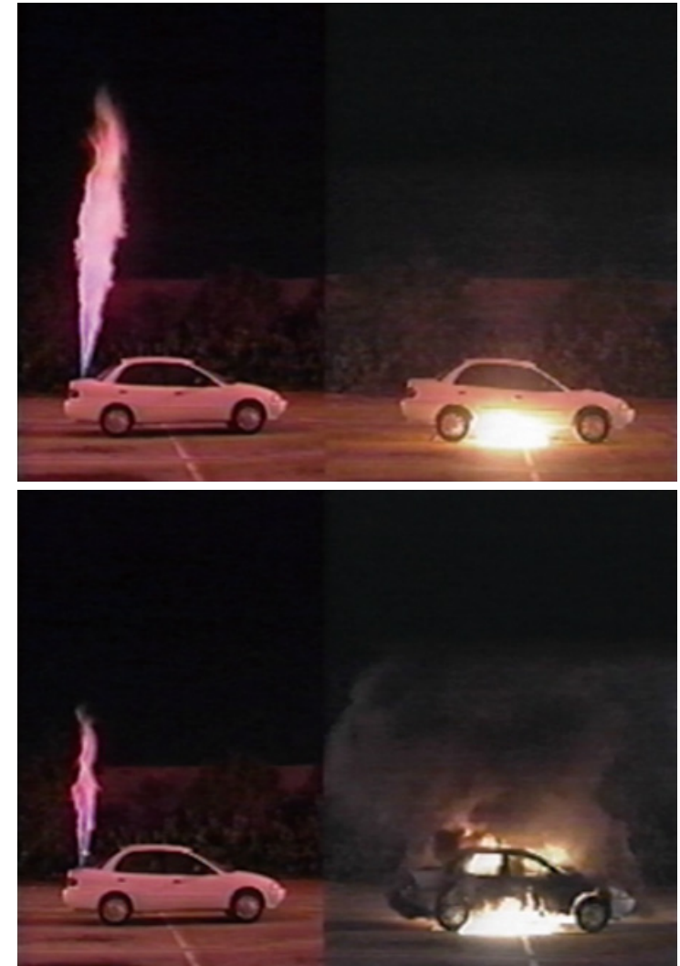
On the left is a hydrogen engine vehicle, and on the right is a gasoline engine vehicle. The top series depicts three seconds after ignition, and the bottom series depicts one minute after ignition. Dr. Michael R. Swain “Fuel Leak Simulation,” University of Miami, 2001.
